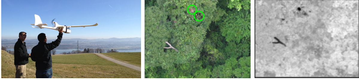
(a) Orangutan nests detection for biodiversity monitoring (UAV-forest). (Left) Conservation drone (image courtesy of conservationdrones.org). (Middle) An arial image captured by the conservation drone, with two orangutan nests highlighted. (Right) The response image generated by a base detector.
