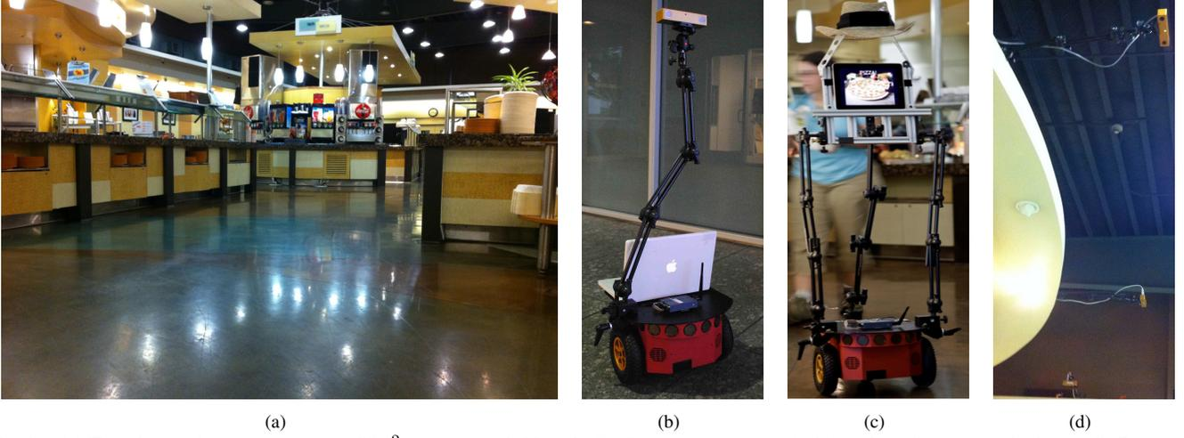
Fig. 3. (a) The robot workspace consists of a 20m<sup>2</sup> area surrounded by a buffet (left), a pizza station (right), and a soda fountain (background). Distance between start and goal was 6m. (b) Old form factor (c) New form factor (d) 3 overhead stereo cameras comprising the tracker.
