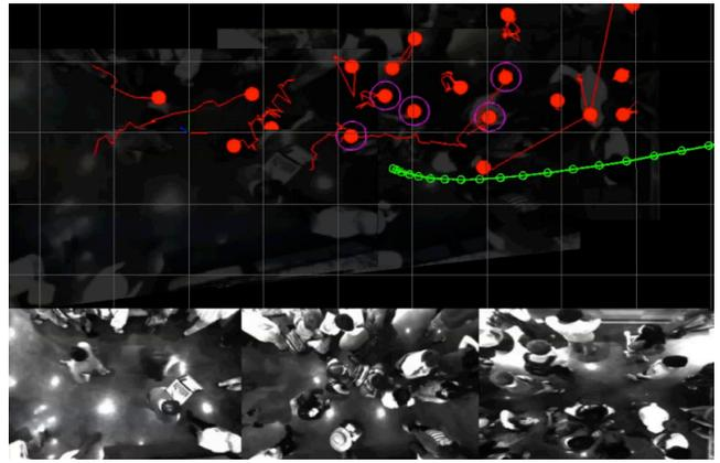
Fig. 4. Robot (wearing sun hat, bottom middle pane) navigating through densities nearing 1 person/m<sup>2</sup>. Green dots are robot’s present plan, red dots are cafeteria patrons, and magenta circles are “salient” patrons (see appendix of [30]). See Section VII for movies of the robot in action.
